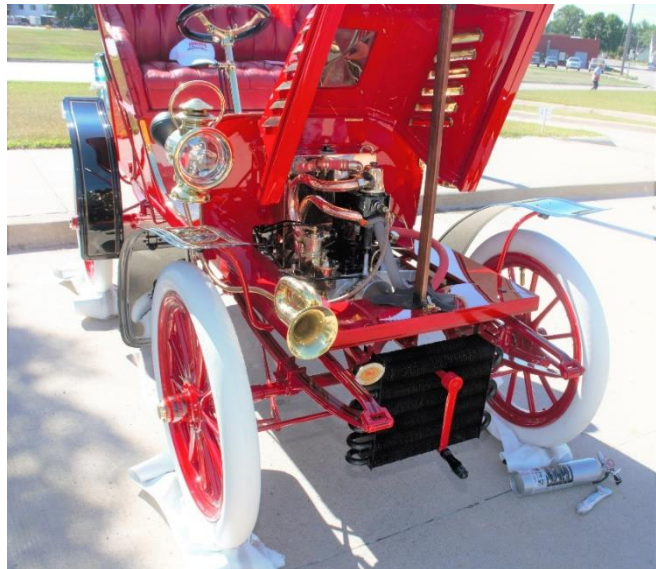
Notice how low the radiator is mounted!
