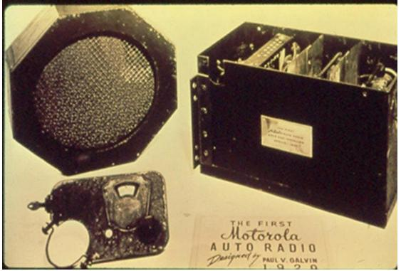
The Tuning panel in the lower left of the picture was mounted to the steering column.
