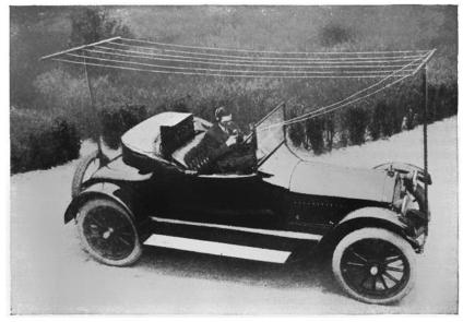
busy installing radio's for their hobby use. The antenna system below looks more like a clothes line. Future designs weaved the antenna into the material top of the car.
