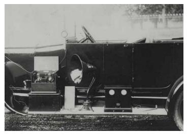
One large problem with the early radios was the different voltages required to operate the tube base radios. The battery operated radios typically needed 3V, 6V, and a third voltage that varied from 22.5 to 135 volts depending upon the manufacturer. A second problem was where and how to mount the antenna for the radio. Early radios had either a single long wire antenna or a "loop" antenna. Amateur radio enthusiast were also
