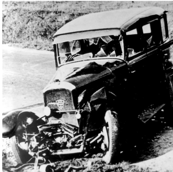
Broken plate glass windshield with jagged edges. Courtesy of Corning Museum of Glass
