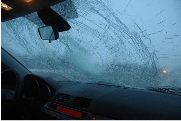
Example of laminated glass breakage. Courtesy of Corning Museum of Glass
