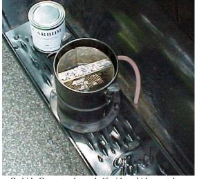
Carbide Generator lower half with carbide crystals.
