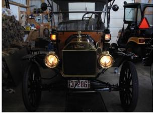
1913 Ford Model T carbide headlamps and kerosene side lamps
