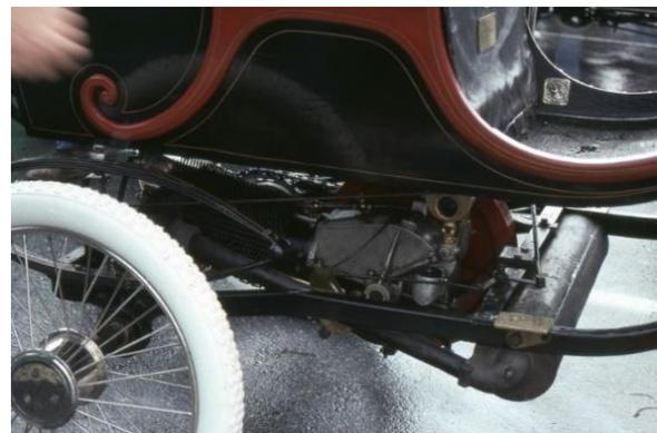
Standard engine placement of the time was beneath the seat
