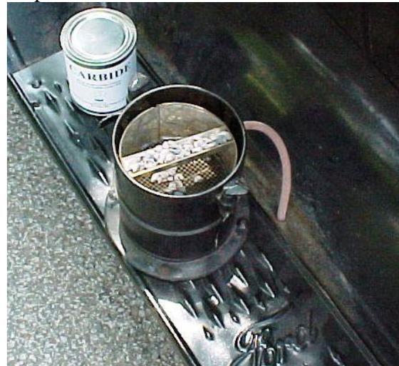
Carbide Generator lower half with carbide crystals.
